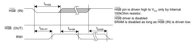
Figure 16. Soft Sequence Processing<sup>[31, 32]</sup>
